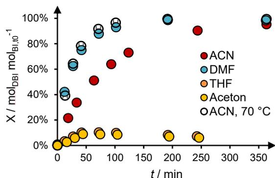
Figure 6: Conversion to DBI for different synthesis solvents ( $K_2CO_3$ ,  $T = 50\text{ }^\circ\text{C}$ ,  $r = 5\text{ mol}_{MI}\text{ mol}_{BI}^{-1}$ , batch,  $n = 3$ )
