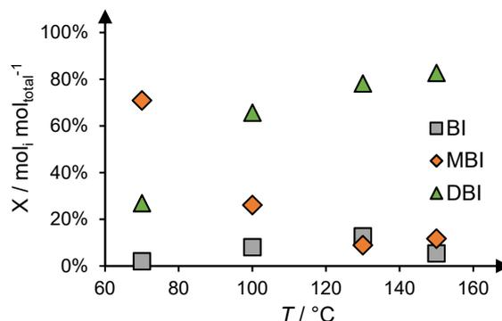
Figure 4: Influence of temperature on the reactor outlet composition in a continuous flow fixed bed reactor ( $K_2CO_3$ ;  $n = 1$  per temperature;  $\dot{V} = 200 \mu\text{L min}^{-1}$ ;  $r = 2.5 \text{ mol}_{AX} \text{ mol}_{BI}^{-1}$ )
