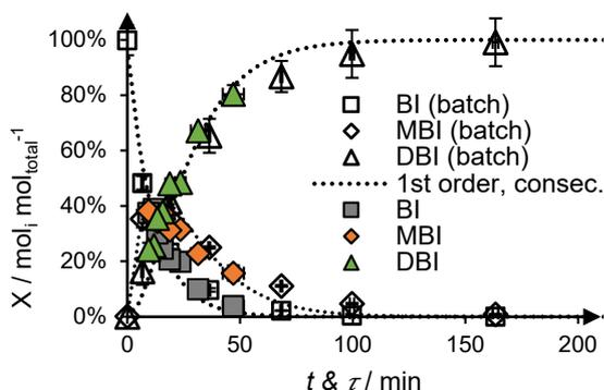
Figure 3: Comparison of conversion to DBI in batch and continuous processing with  $K_2CO_3$  as basic reagent ( $r = 5 \text{ mol}_M \text{ mol}_{BI}^{-1}$ )
