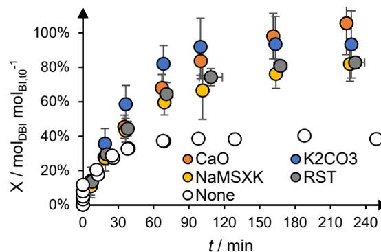
Figure 5: Conversion to DBI with none and a selection of basic reagents from the groups of metal oxides, activated carbon, zeolites and alkali ( $r = 2.5 \text{ mol}_M \text{ mol}_{BI}^{-1}$ , batch,  $n = 3$ )
