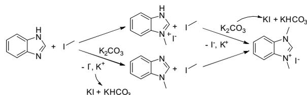
Figure 1: Assumed reaction scheme of the 2-step synthesis of 1,3-methyl-benzoimidazol-3-ium iodide (DBI) in the presence of a solid base (K<sub>2</sub>CO<sub>3</sub>) and methylene iodide (MI). Intermediate: 1-methyl-1*H*-benzoimidazol-3-ium iodide (MBI)
